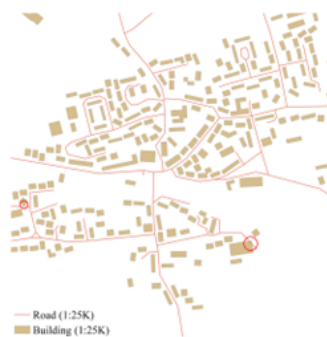
e. OSGB - Generalized Building features from the AGENT model and Road features of the target scale (input to the CartACom model)
