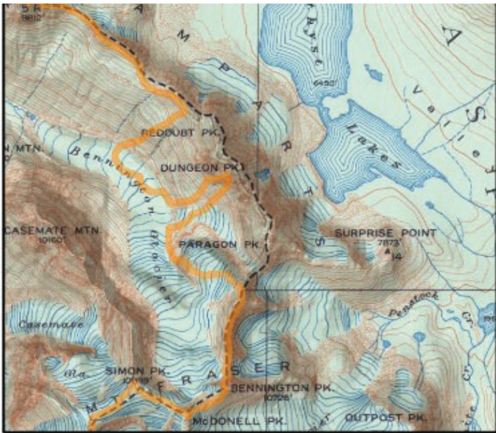
Figure 2. NRCan's watershed boundary (in orange) overlaid on top of the original 1:62,500 topographic maps sheets created from the 1913-1924 survey. The original surveyed watershed line is shown as a dashed black line.
