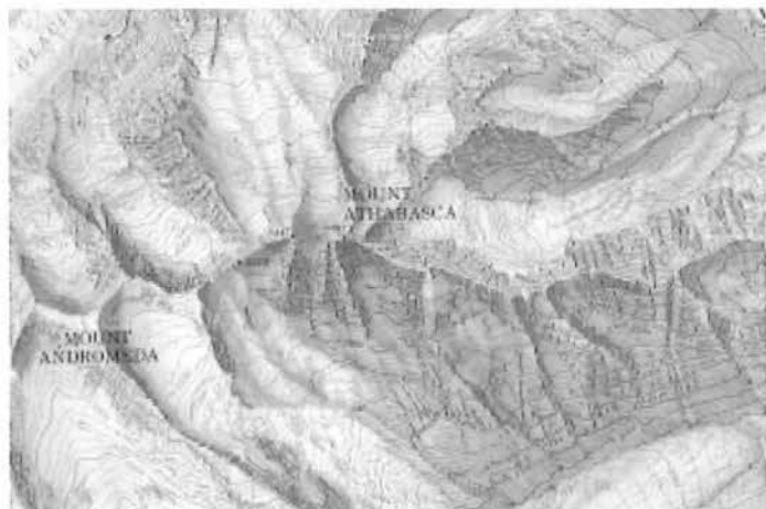
Figure 2: Columbia Icefield, 1:50,000, contour interval 20 metres (100 metres on bedrock), 1980.
